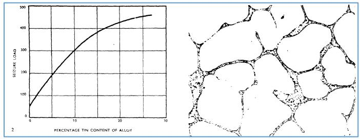
Figure 1. Above: The effect of the addition of tin to aluminium on the seizure resistance. Figure 2. Right above: Structure of 20% aluminium-tin as cast and unrolled.
