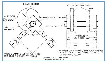
Figure 5. Layout of loading system for machine in Figure 4.
