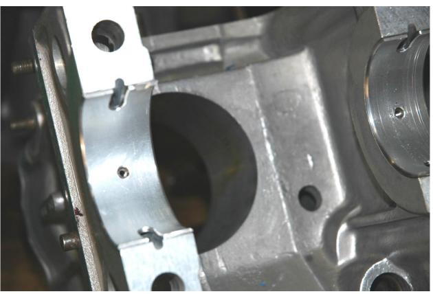
.An Alutin bearing shell installed on a Javelin front main bearing support.
