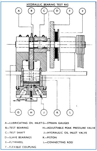
Figure 7. Arrangement of test head on machine in Figure 6.
