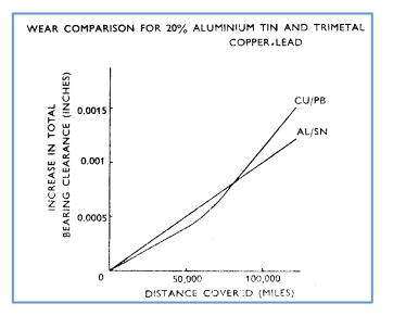
Figure 8. Above: Comparative wear of bearing materials.
