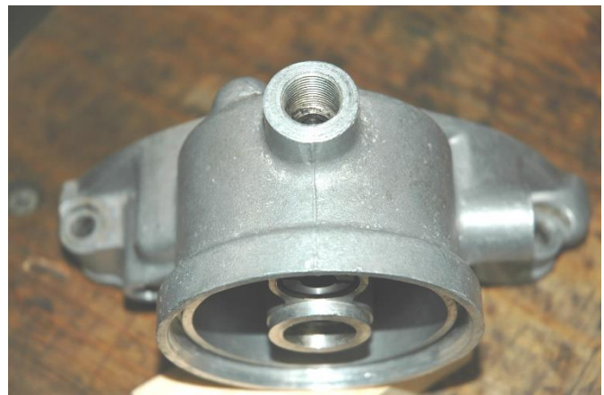
Figure 5: Showing the enlarged outlet port.
