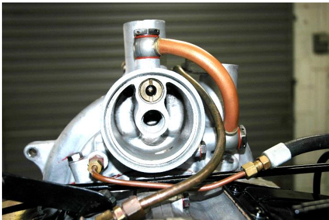
Figure 6: Showing an installed oil transfer pipe.
