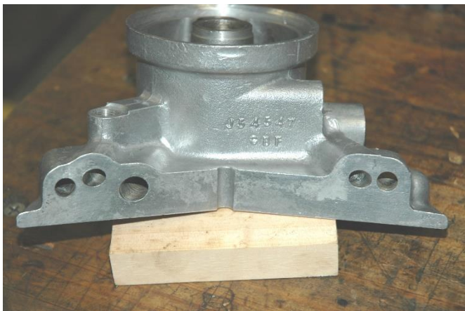
Figure 3: The oil galleries to be enlarged.
