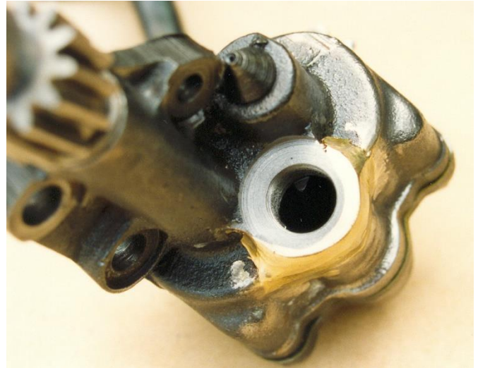
Figure 11: Illustrates built up pump body.
