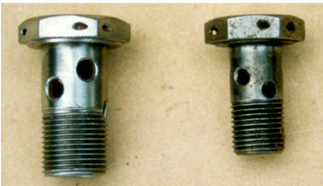
Figure 9: Comparison of larger banjo bolt.
